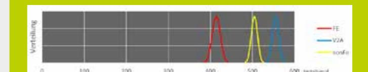
As part of the manufacturer validation, trigger signals for FE, V2A and nonFe are recorded and checked for the presence of a normal distribution. The diagram of the distribution can be seen in the certificate.
